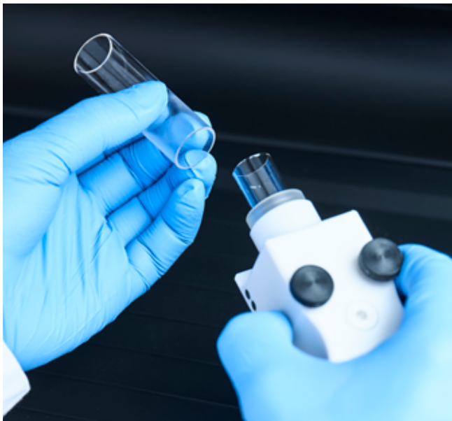
Modular demountable torch (V Shuttle Torch)
