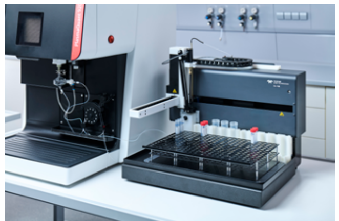
Autosampler Oils 7400 by Teledyne CETAC Technologies
