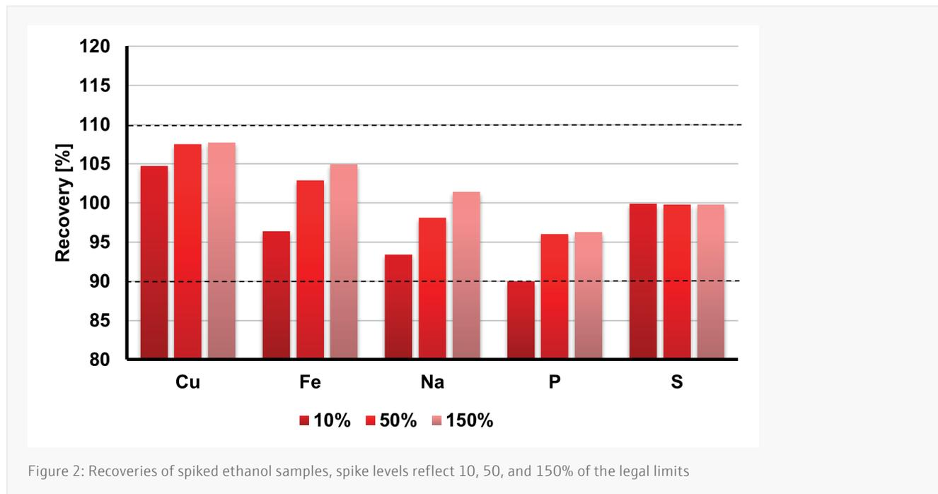
Figure 2: Recoveries of spiked ethanol samples, spike levels reflect 10, 50, and 150% of the legal limits
