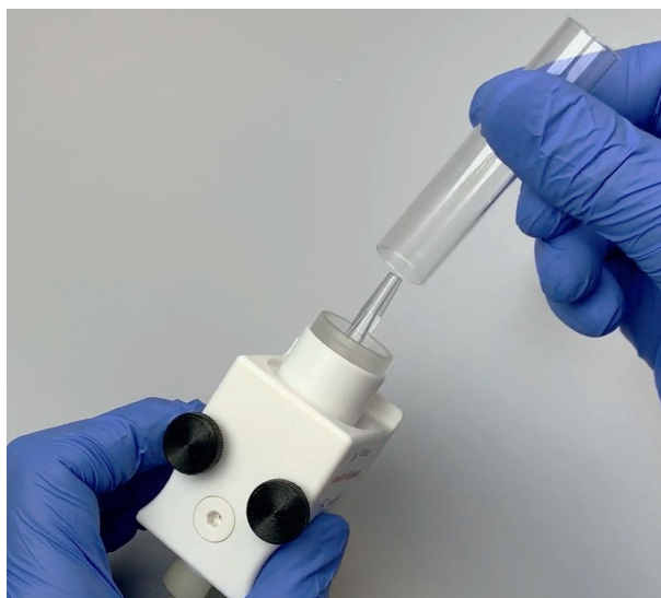
Fig. 37 Video: Cleaning the demountable torch (available in the online help)
