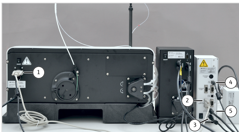
Fig. 27 Connect the control unit of the switching valve
