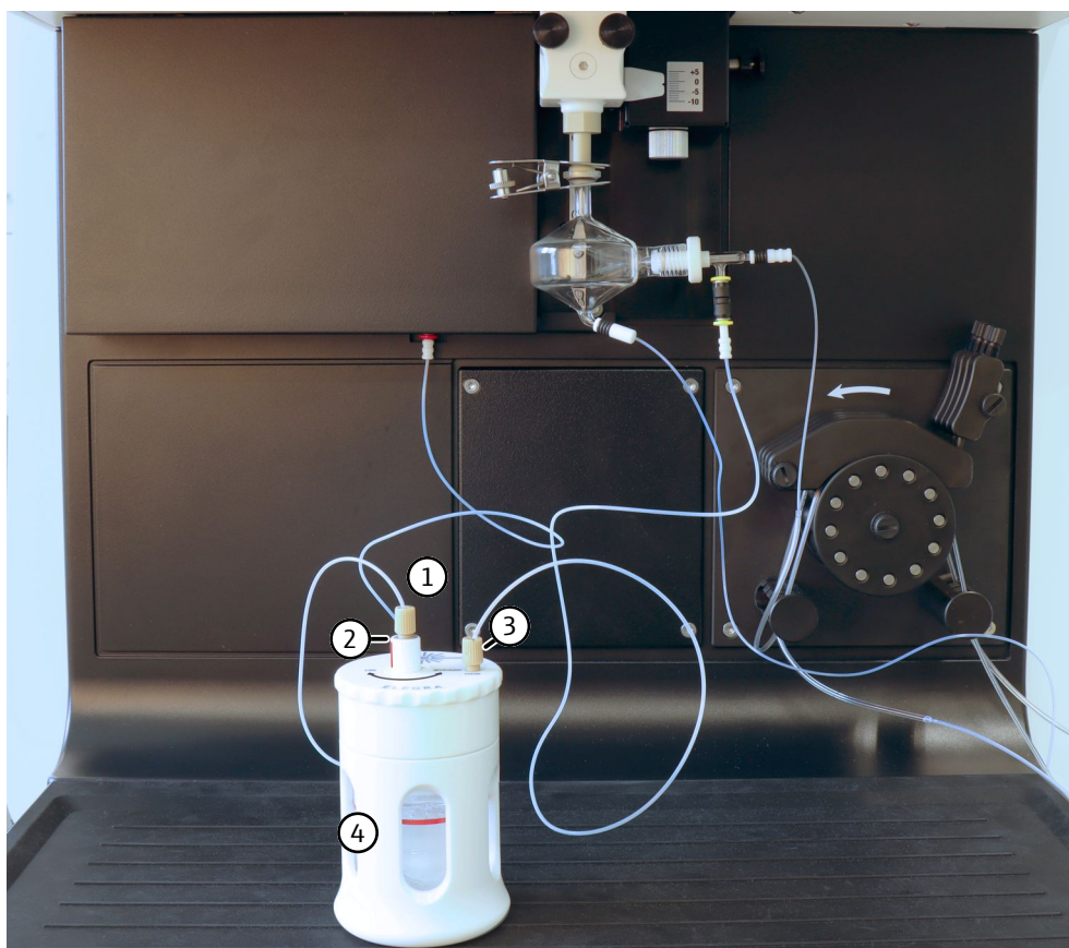
Fig. 33 Installing the argon humidifier
