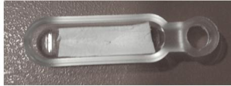
**Fig. 24 Quartz boat with correctly inserted quartz fleece**
