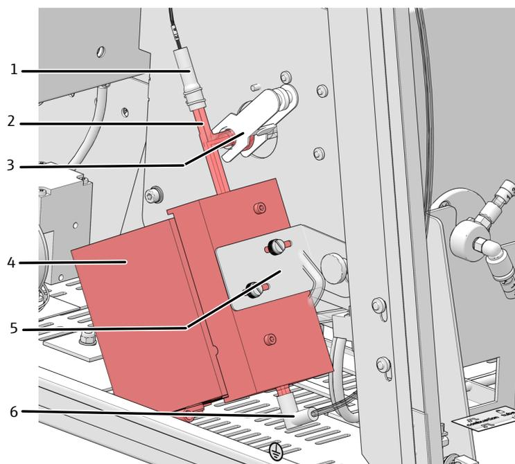
**Fig. 12 Peltier cooling block with T-connector**
