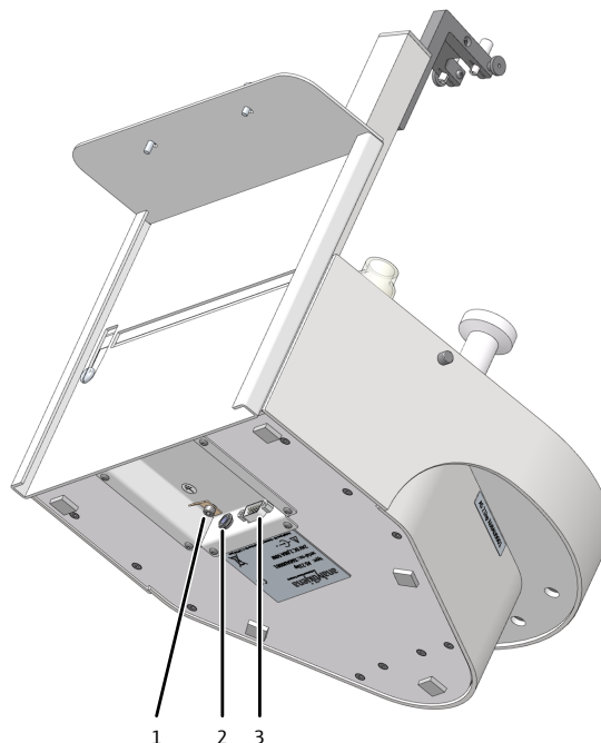
Fig. 21 Connections on the bottom of the autosampler
