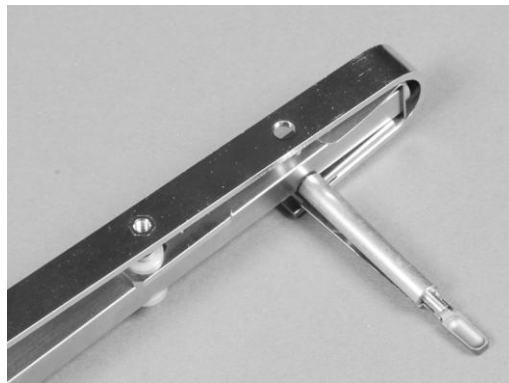
Fig. 5 Tweezers with sample platform
